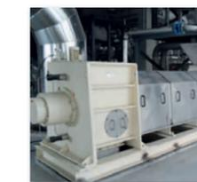
The VetterTec screw press is used to pre-dewater corn germ and corn fibre in front of the dryer. In all our screw presses the screw, screen and cage are precisely machined together. The entire mechanical design is very strong. Both, the machining and design, is ensuring best and constant pre-dewatering results and minimizes the energy demand in the dryer.
